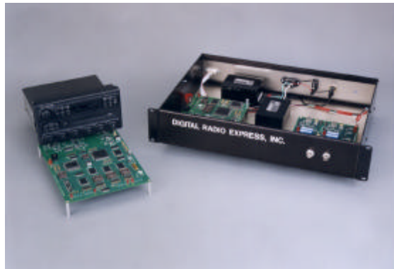
Figure 2. DRE FM IBOC Prototype Hardware – receiver (left) and exciter (right)
