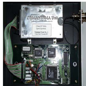
Diagram 4 – Inside of IP-wireless terminal
