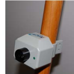
(S1) Super sonic sensor unit on stick to detect obstacles
