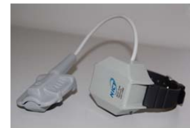
(S3) Sensor unit on watch for pulse, SpO2, and body temp.
