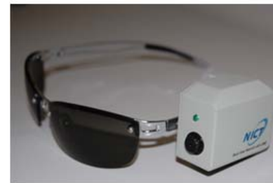
(S1) Camera unit on glasses for discrimination of traffic signals
