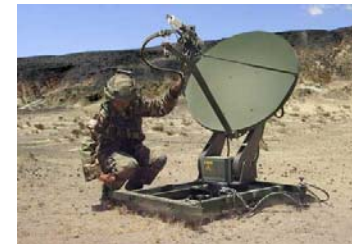
Remote VSAT Stations
